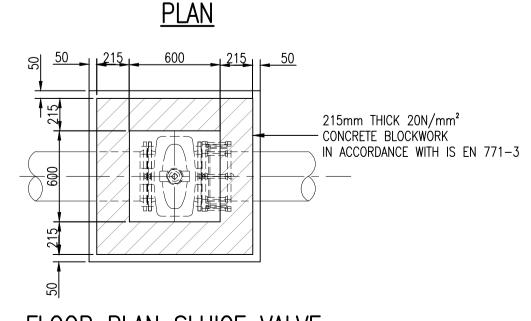
FLOOR PLAN SLUICE VALVE CHAMBER (BLOCKWORK
